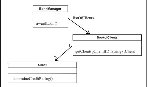
The system shown above is driven by the BankManager class. The awardLoan() method is invoked, either via the interface or from another method. This method is intended to accept or reject a loan application.
