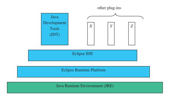
Lots of other plug-ins are available to support additional tools (style-checking, testing, GUI design etc.) and languages (including C/C++).
