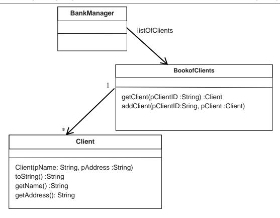
In this system a BankManager class maintains a 'map' of clients. Client objects can be added by the addClient() method which requires an ID for that client and the client object to be added. Clients can be retrieved via the getClient() method which requires a ClientID as a parameter and returns a client object (if one exists) or generates an exception (if a client with the specified ID does not exist).
