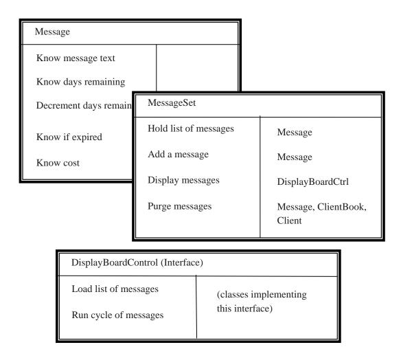
What we want to 'test' here is that messages can be created, added to the MessageSet and displayed on the display.
