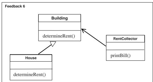
By showing determineRent() in House we are showing that this method is overriding the one defined in the superclass (Building).
