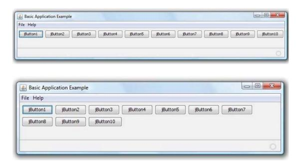
A flow manager can be created with various properties to define the justification of the object (centre, left or right) and to define the horizontal and vertical space between objects.
