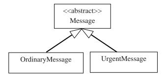
However in this case there are no unique features of an ordinary message – messages have an associated cost, the cost and text can be obtained and new messages can be created. All this is true for urgent messages. An urgent message is just the same as an ordinary message where the text and the cost has been changed slightly. Thus UrgentMessage is a type of Message and can inherit ALL of the features of Message with the cost and text methods being overridden.
