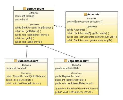
Thus given the diagram above NetBeans would create four classes, three of which would automatically be placed in an inheritance hierarchy. Method stubs would be created for each of the specified methods and while the code inside each method would still need to be written the constructor for CurrentAccount would automatically invoke the constructor for Bank Account passing the parameter pBalance upwards.
