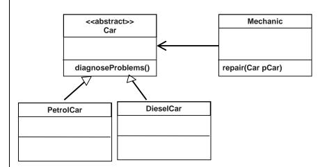
Here Mechanic is directly interacting with Car. In doing so it can interact with any subtype of Car e.g. Petrol, Diesel or any other type of Car developed in the future e.g. (Electric). These are all different (different shapes) and yet Mechanic can still interact with them as they are all Cars. This is polymorphic.
